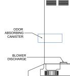
11) Move the canister all the way to the back and then lower the canister over the blower discharge. Shift the canister front to back and left to right to make sure that the blower discharge and canister have fully engaged.
