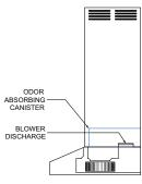
12) With the gasket side facing down, nest the smoke trapping filter element into the pocket that forms the top of the odor absorbing canister. The filter may have a rectangular base so rotate as necessary.
